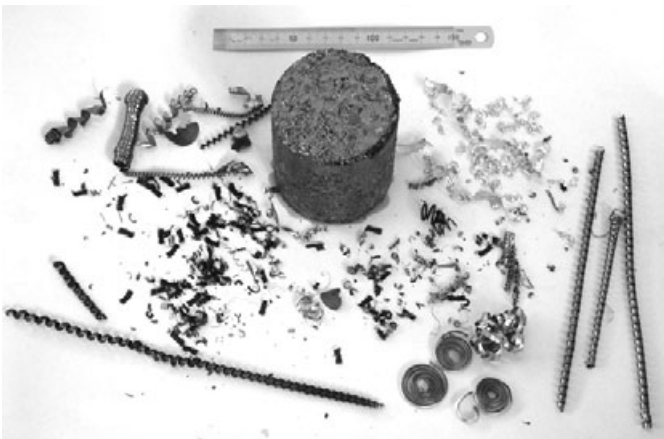
FIG. 3—Photo of various types of swarf, including a block of compressed swarf.
